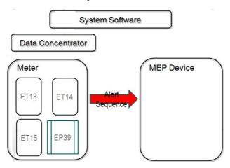
3) Upon detecting the alert sequence from the OSGP device, the MEP device polls the alert bits in ET13.
